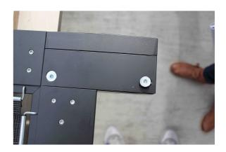
It might be necessary to add the linking device for a better connection between 2 units in case of configuration  $90^{\circ}\,$
