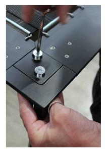
Tighten the screws with the Allen key
