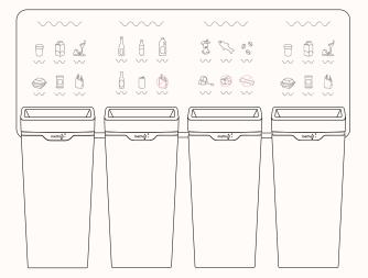
4 bins connected by HD connectors with signs OW 1560mm OD 350mm
